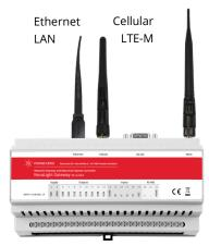
our technical support. Different parameters are required: an APN with an optional username and password and a PIN code. The platform automatically recognizes the name of the network operator, the quality of the cellular signal, the technology used, the IMEI and IMSI number.
